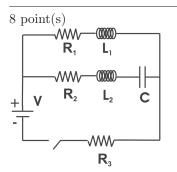
Consider the circuit shown in the figure above. The switch has been open for a very long time, and then we close it. Rank the magnitudes of the currents through resistors  $R_1$ ,  $R_2$ , and  $R_3$ , from greatest to least, in the instant right after we close the switch. Assume that  $R_1 > R_2 > R_3$ .
