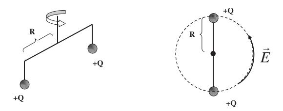
a) (5 points) We start out with everything stationary and with no external fields. Then, we turn on a magnetic field of strength **B** pointing upward (out of the page from the top-down view). It takes some time **t** for the field to ramp up. While the magnetic field is changing, there's a voltage induced on the loop of radius **R** that includes both charges. What is that voltage?
