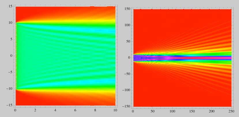
Fresnel zone shows shadow boundary, diffraction fringes
