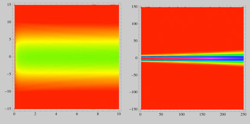
Beam smoothly spreads out with distance
