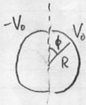
Conducting cylinder of radius  $R$  split into two halves held at  $-V_0$  and  $+V_0$ . Let's hack away at  $V$  (everywhere)
