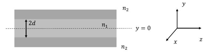
An optical fiber is basically this setup, but with a cylindrical geometry. The inner and outer layers are referred to as the core and cladding, respectively. Note that in general we have  $n_1 > n_2$ . The ray optics view of this system is that the light propagates down the center, totally internally reflecting off of the two interfaces – and total internal reflection requires that you be going from high index into low index.
