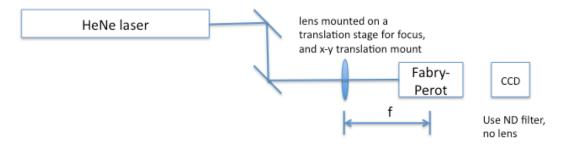
Use mirrors to get the beam level and straight to the table holes, then position your interferometer and camera at the same beam height. The lens should be mounted on a
