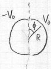
Conducting cylinder of radius  $R$  split into two halves held at  $-V_0$  and  $+V_0$ . Let's look away at  $V$ .
