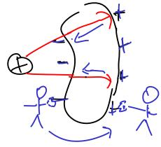
I pick up the charges and move them to the other side of the conductor causing a steady current to flow (acting as a battery)
