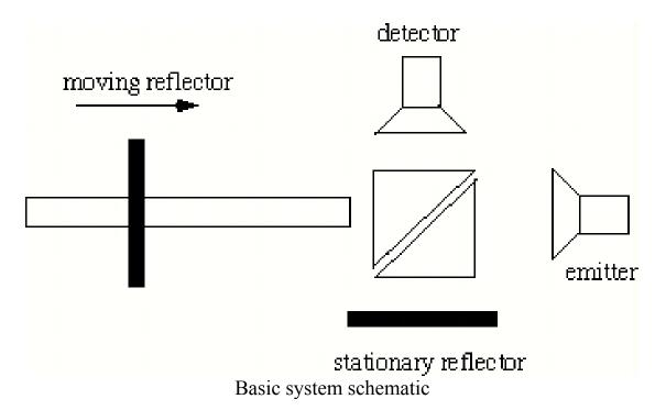
With this apparatus we can capture a fringe pattern in time. The detected field is the sum of the fields in the two arms. If we assume that the beamsplitter is 50/50, we can calculate the fringe pattern that we can expect to measure. The field entering each arm can be written as
