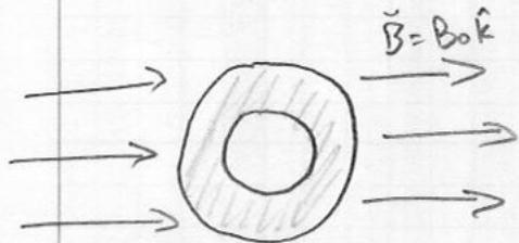
Consider a spherical shell of material with permeability  $\mu$  and inner and outer radii  $R_i$  and  $R_o$ .
