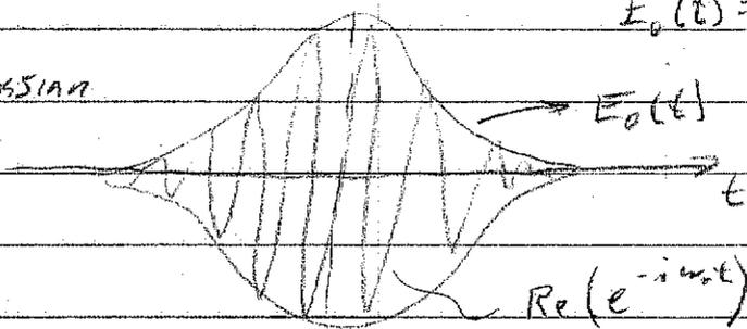
Any modulation in the time domain requires a mixture of frequencies. Use Fourier transforms to get spectrum:
