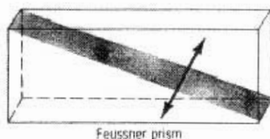
FIGURE 13-13. A Feussner polarizer. The optical axis of the birefringent material is normal to the slab of material as shown by the arrows.
