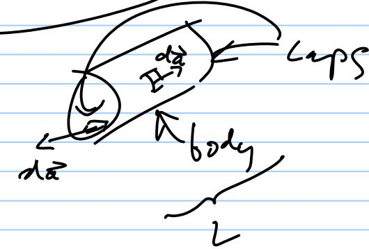
body :  $\int_{\text{body}} \vec{E} \cdot d\vec{a} = \int_{\text{body}} |\vec{E}| |d\vec{a}| \cos 0^\circ = E \int_{\text{body}} |d\vec{a}|$
