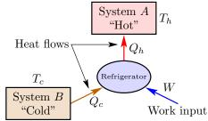
Since all of the heat flows and the work flow are reversed relative to the heat engine, we'll reverse the sign conventions to make them all positive. The analysis of the process is much the same as for a heat entine, but we need a slightly different definition of performance:
