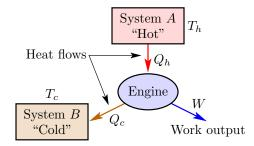
The idea is that the engine, which is supposed to be unchanged by the net process, absorbs some heat  $Q_h$  from a hot system and uses that to produce some useful work output W, while dumping a portion  $Q_c$  of the heat into a cold system. Here the terms "hot" and "cold" refer to the relative temperatures of systems A and B.
