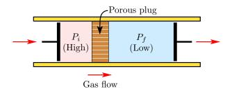
Consider a portion  $V_i$  of the gas on the left passing through the plug and having volume  $V_f$  at pressure  $P_f$  afterward. The process is adiabatic (no heat flow), so the change in energy of the gas is due entirely to the work done by the pistons during the flow. The pressure is constant on both sides, so the work done by each piston is a simple PV product:
