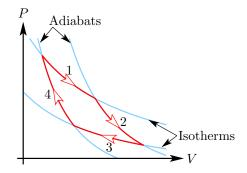
Recall from an exercise we did long ago that adiabats are steeper than isotherms in the pressure vs volume diagram, because heat transfer in isothermal processes reduces pressure changes.
