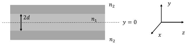
An optical fiber is basically this, but with a cylindrical geometry. The inner and outer layers are referred to as the core and cladding, respectively. Note that in general we have  $n_1 > n_2$ . The ray optics view of this system is that the light propagates down the center, totally internally reflecting off of the two interfaces – and total internal reflection requires that you be going from high index into low index.
