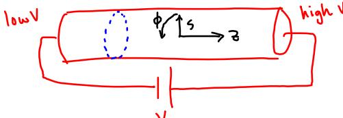
You apply a voltage  $V$  to it, and current flows. Let's assume constant resistivity, this leads to a constant E-field along wire.
