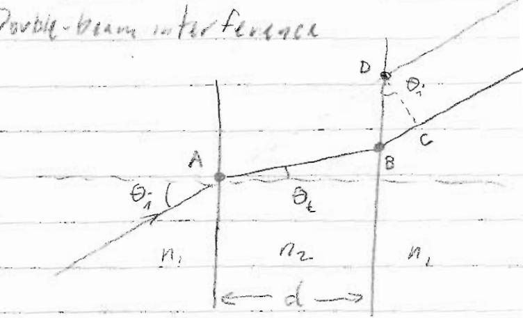
Suppose we introduce a tilted window into one arm of an interferometer. What is the phase shift?
