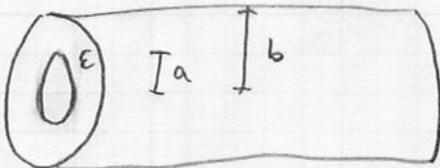
Imagine taking a parallel-plate waveguide and rolling it up. It'll give you a coax cable with free space from  $a < r < b$ , or if you prefer, some dielectric  $\epsilon$ .
