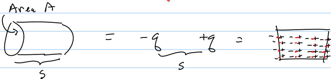
This is equivalent to dipole moment  $qS = \underline{P}AS$
