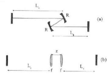
Assuming the following parameters that are typical of a Kerr-lens mode-locked laser:  $L_1$  = 400mm,  $L_2$  = 1000mm, f = 50mm. Using the ABCD code, set up the ABCD matrix and make a plot of the stability parameter as a function of the curved mirror separation z. Also plot of the cavity mode size at each end of the resonator vs. z.
