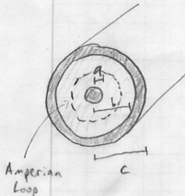
Coax cable. Interior wire has radius  $a$ . Return sheath has inner and outer radii  $b + c$ .
