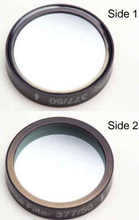
Semrock DAPI Exciter After > 1000 hrs
